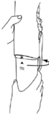
Figure 3: Hold the unit and rotate the skirt in anti-clockwise direction to take off the skirt.
